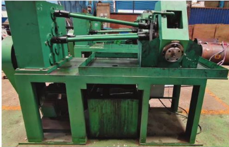
Extruded Finning Machine 3 Nos (Up to 16 Mtr Length)
