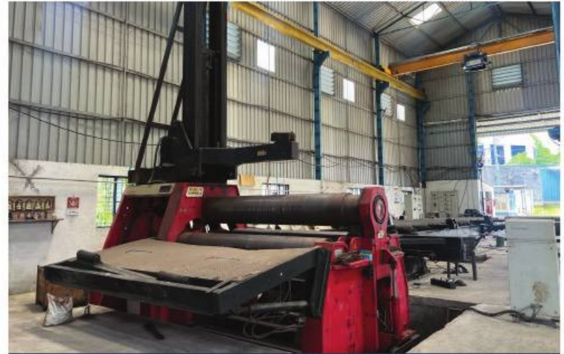
CNC Fully Automatic Rolling Machine Thickness : 85 mm / 3 Mtr width / 6Mtr Dia
