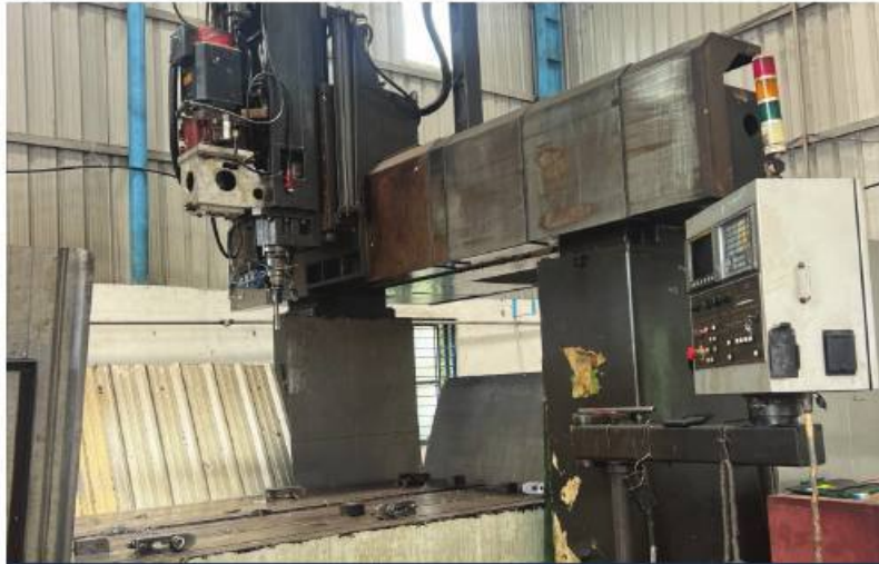
VMC Drilling Machine Thickness : 300 MM / 1.9 Mtr
