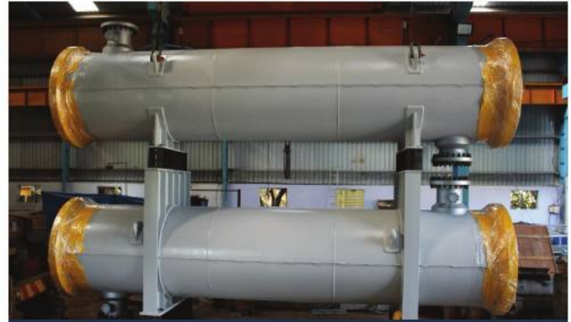
Client Name : IOCL Panipet Type : Stacked Exchanger / 35 Ton
